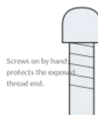
Rod / stud end cap — screw-on thread protector, moulded LDPE, not to scale
