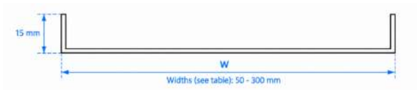
Light Duty Cable Tray — cross-section and base detail, dimensions in mm, not to scale
